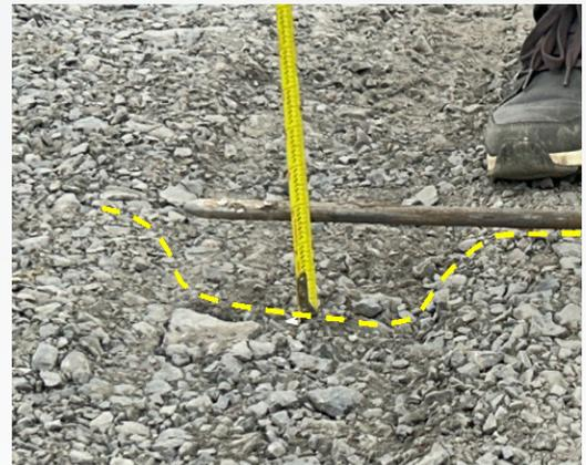
Section 2 - Biaxial Grid 1: 60mm rut
