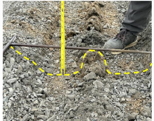
Section 3 - Biaxial Grid 2: 100mm rut
